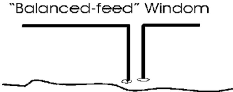
Properly installed Windom antennas have impedances in the 400-600 ohm range at resonant frequencies. Depending on the installation, a Windom antenna may have reasonable impedances at several harmonically related frequencies.
