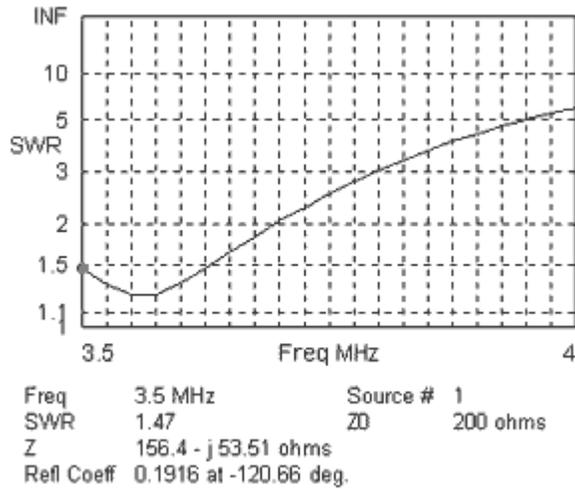
**Above is an SWR Plot of full-wave horizontal loop at 60 feet, resonant at 3.54MHz while using a DX Engineering 4:1 balun. Below is 40 meter SWR.**
