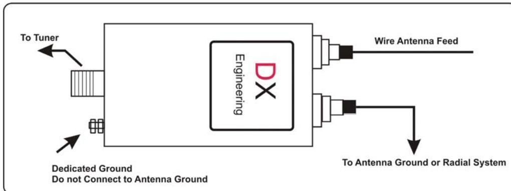
**Long-wire Feed using a 4:1 Balun. The antenna ground side should be attached to a radial system as with a vertical antenna.**
