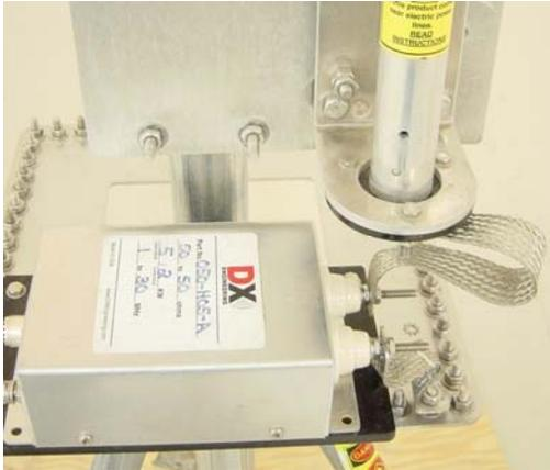
**Figure 1 Insulated Balun System for use with Hustler Antenna and Radial Plate.**
