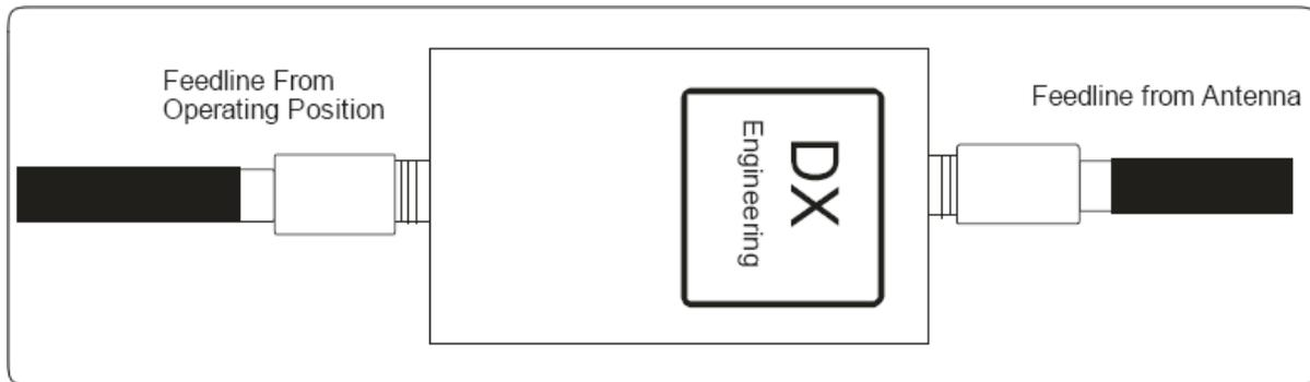
**Feedline Current Choke: Use with any vertical or horizontal antenna that is coaxially fed.**
