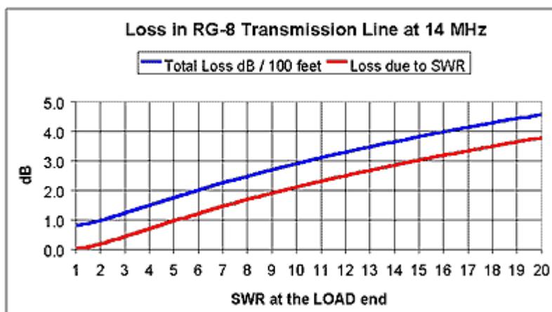
**Why you don't want to use coax when the SWR is high. For each 100 feet of coax, you lose half your power at an SWR of 10:1. At frequencies higher than 14MHz, it's worse. For higher loss coax like RG-58 or RG-8X it is worse, too. Plus, the SWR shown here is measured at the antenna, not at the radio where it would measure significantly lower but still would eat up just as much power.**
