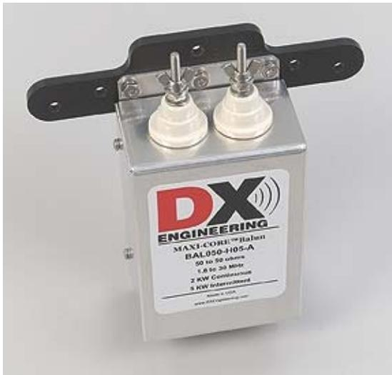
The optional, formed plastic piece shown on the back of the DX Engineering balun allows it to be mounted on the wire element and removes the load of the balun and feedline from the element wire ends, which will keep them from breaking in most installations.
