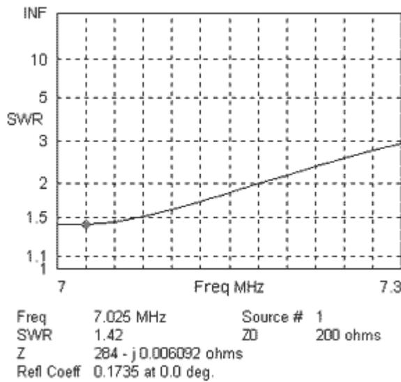
**The plots above show with a DX Engineering 4:1 balun and reasonably good coax, you can operate a loop over most of 80 and all of 40 meters. This system is generally good on 80, 40, 20, 15 and 12 meters.**
