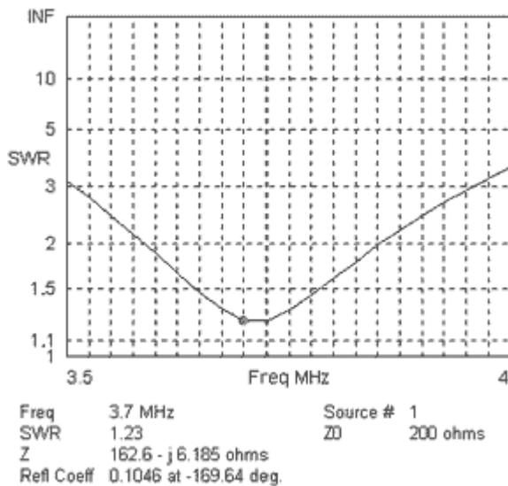
**Typical SWR Plot of full-wave horizontal loop at approximately 60 feet above average ground using DX Engineering 4:1 balun. Operation is safe for balun and coaxial feedline over the entire band.**
