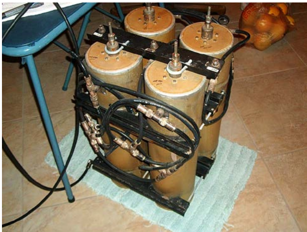
These are the cavities for the repeater, Looks like a plumber's nightmare.
